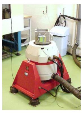
**3 shakers machines** (up to 13kN) IEC 60068-2-6, IEC 60068-2-64, ISO 16750-3
